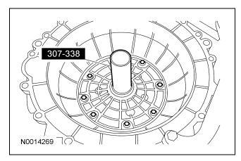
114. CAUTION: Do not damage the fluid pump gear O-ring seal when installing torque converter.
